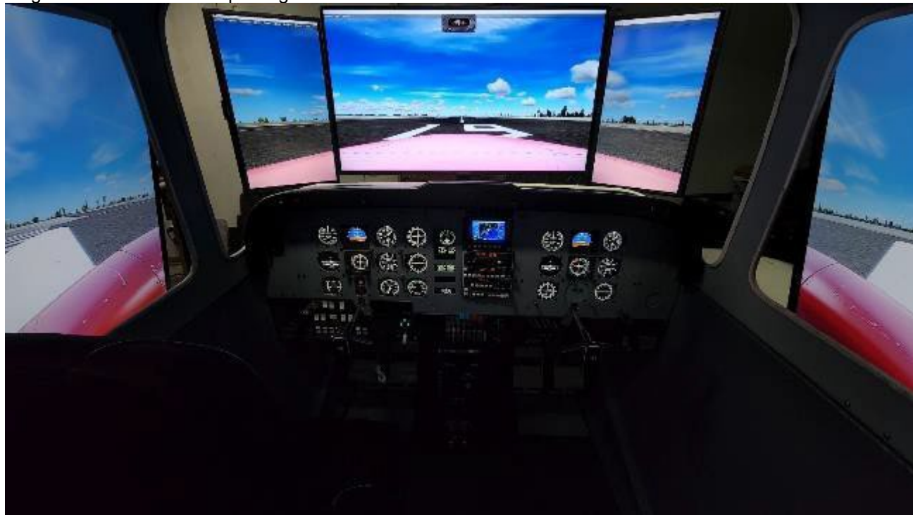
Image 23: ATD Panel in Piper Aztec Configuration with optional Co-Pilot System, XCS55A, XNS530W and MegaRadioStack Avionics package.
