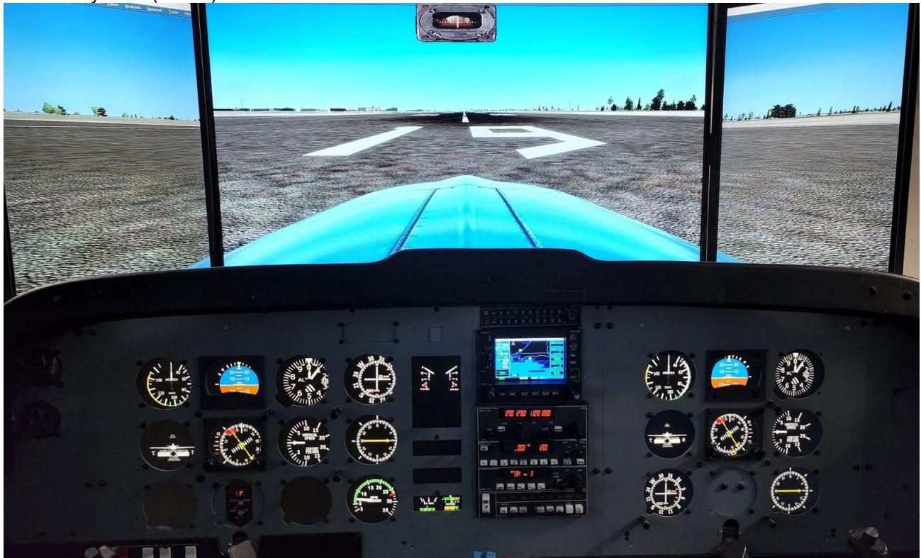
Image 37: Detail view of ATD Panel with Optional Co-Pilot Package, Optional MegaRadioStack Avionics and XCS55A system. (PA-38)
