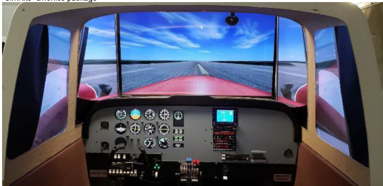
Image 22: ATD Panel in Piper Aztec Configuration with optional Enhanced Visuals System and optional TRC “SimKits” avionics package
