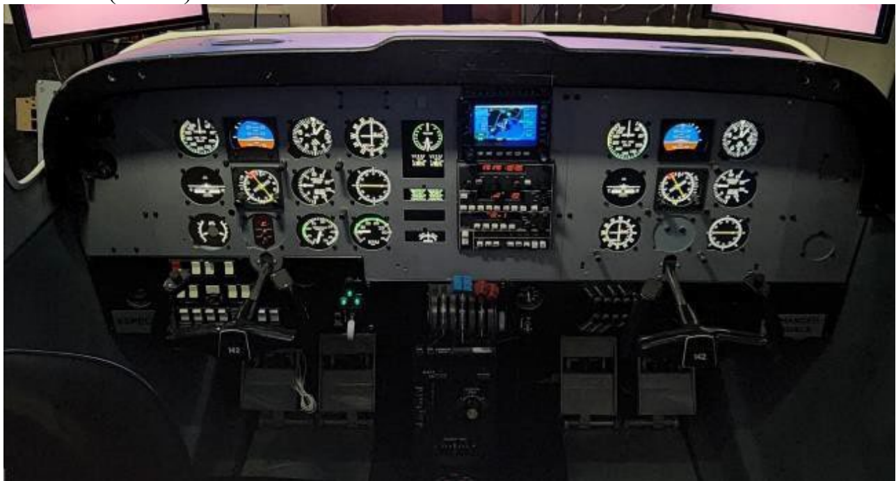
Image 7: Optional Co-Pilot Package, KA-51B, KX155, KR87, KT76C, KFC150 GNS530. (PA-23)
