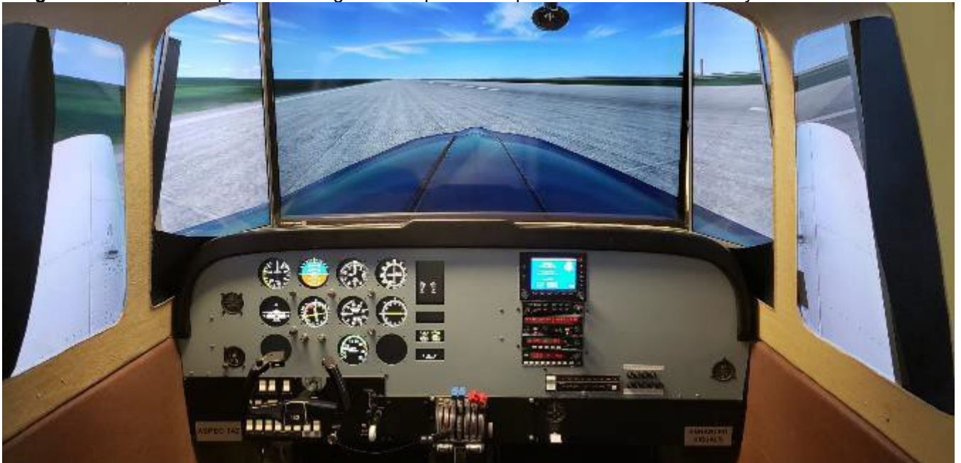
Image 35: View of PA-38 panel with magnetic compass and optional Enhanced Visuals System
