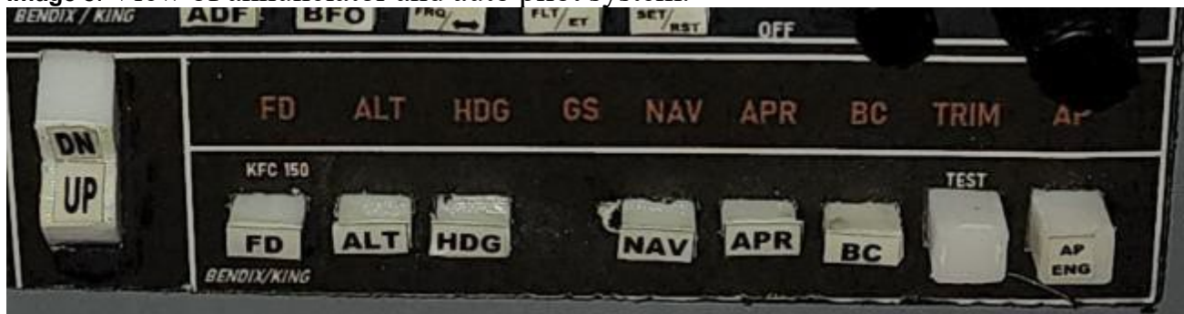
Image 8: View of annunciator and auto pilot system.
