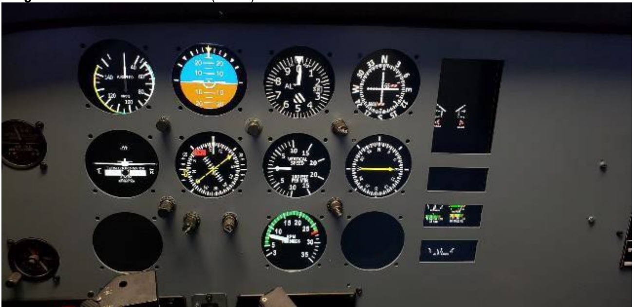
Image 36: Detail view of ATD Panel (PA-38)
