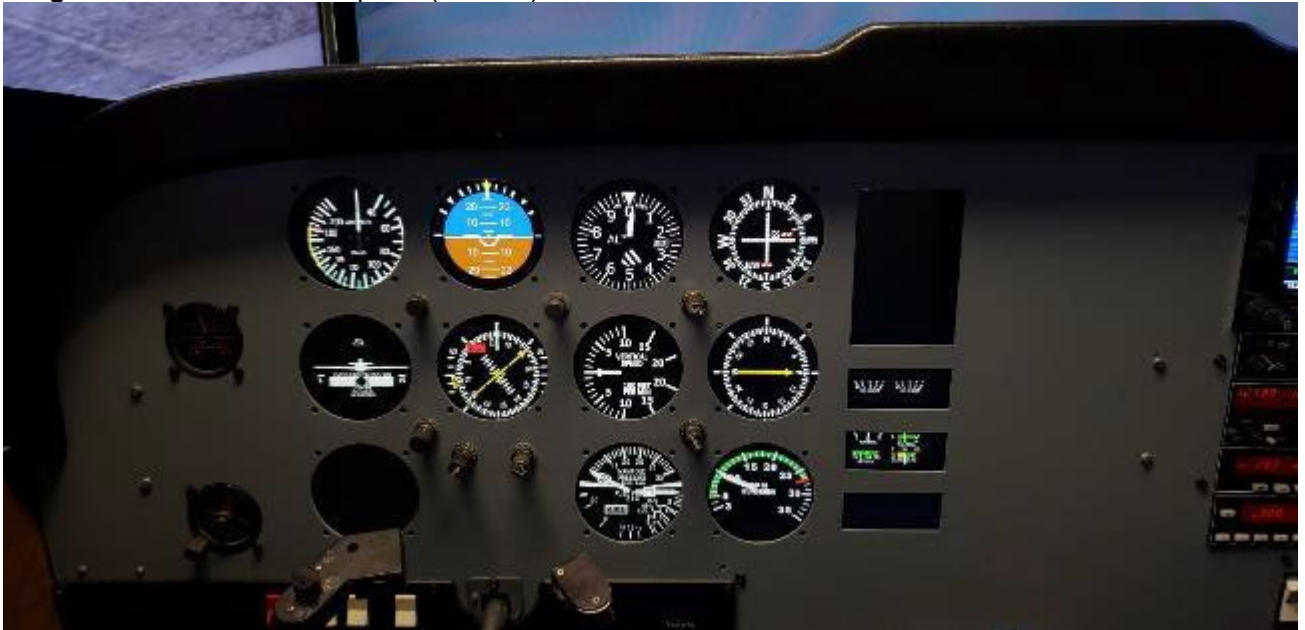
Image 39: Detail view of ATD panel (PA-28R)
