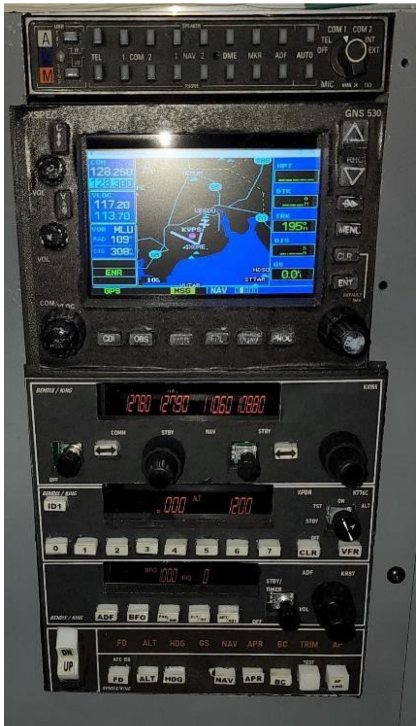
Image 5: Detail view of Alternate Avionics Panel “MegaRadioStack” KX155, KR87, KT76C and KFC150 below an alternate “XSPEC” GNS530. KMA24 Audio Panel.
