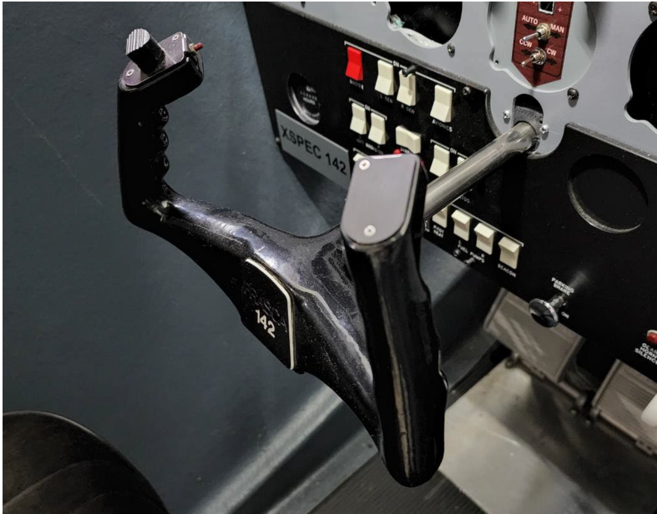
Image 12: Control Yoke showing yoke mounted switches. (MEL)
