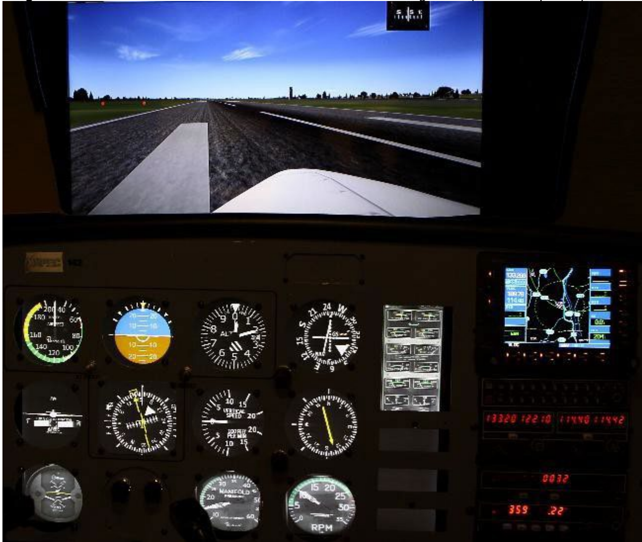
Image 18: Detail view of ATD Panel in Beechcraft Duchess BE-76 Configuration (Pilot's Perspective)
