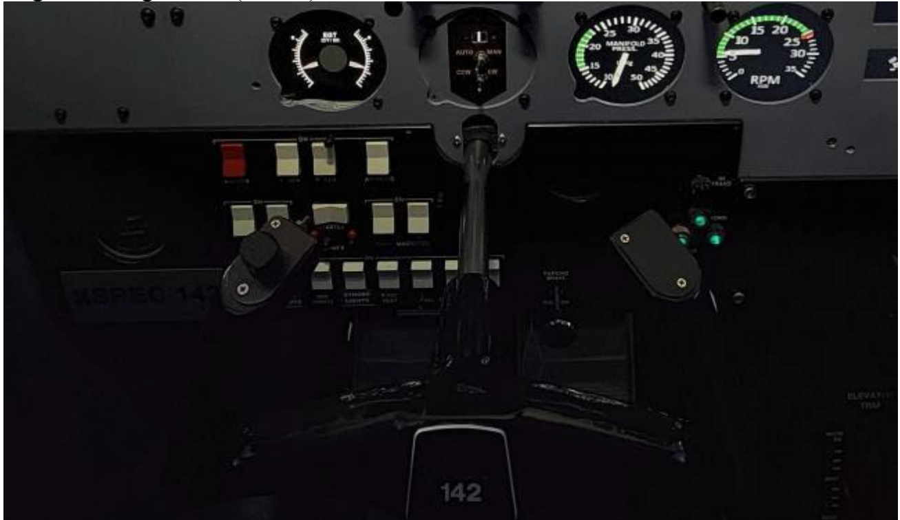
Image 6: Engine start panel and switches with optional KA-51B Slaving Panel in Multi-Engine Configuration (PA-23)
