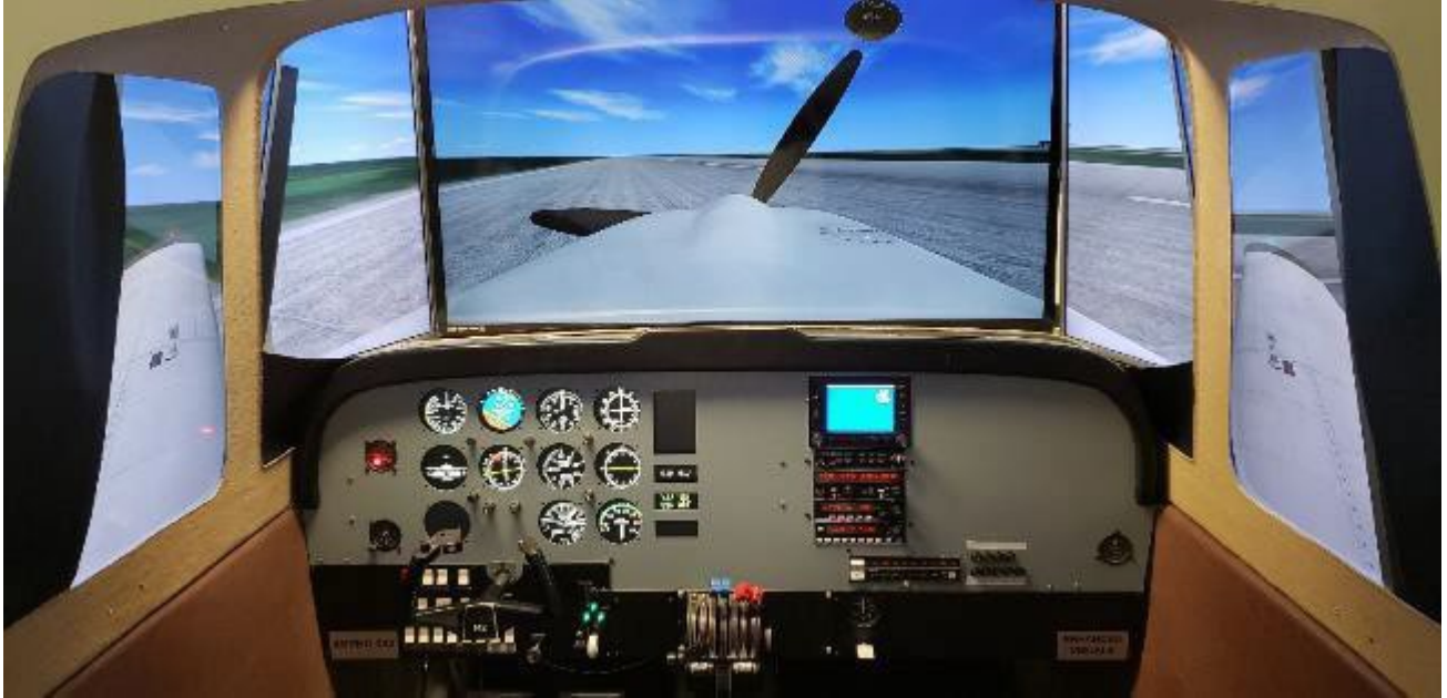
Image 38: View of PA-28R panel with magnetic compass and optional Enhanced Visuals System in Optional Double Wide Enclosure
