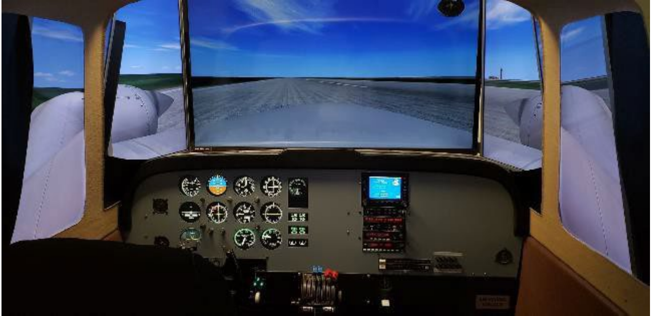
Image 33: View of PA-34 panel with magnetic compass and optional Enhanced Visuals System.
