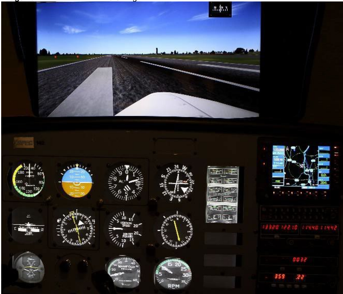
Image 40: ATD Interior in BE-76 Configuration.
