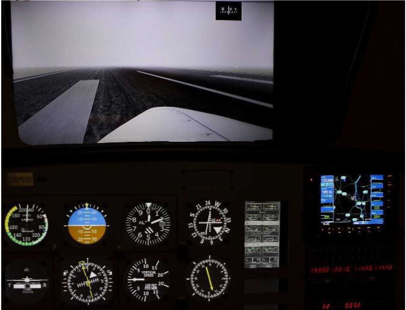
Image 41: ATD Interior in BE-76 Configuration
